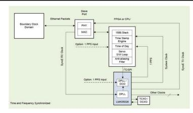
Figure 1. The LMK05028 Working as a Slave Clock.
