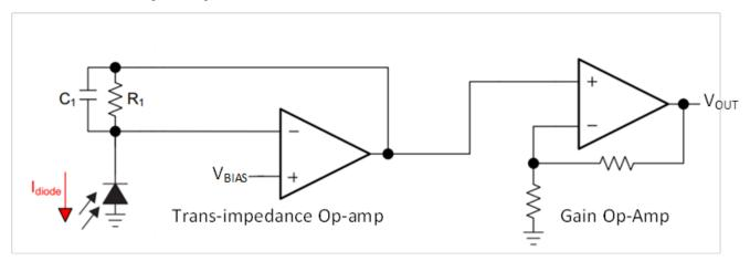
Figure 2. Optical Smoke Detector Working Principle
