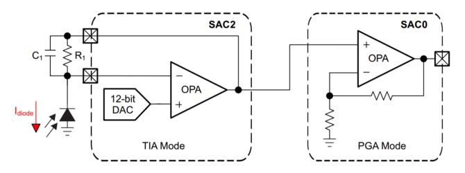
Figure 3. Using Smart Analog Combo Modules for an Optical Smoke Detector
