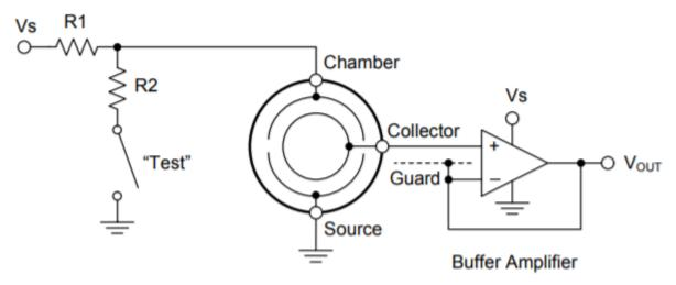
Figure 1. Ionization Smoke Detector Working Principle
