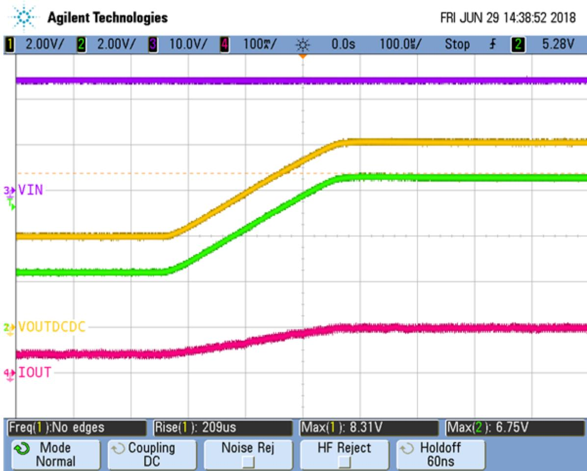
**Figure 4. The LMR33630 Tracking the Up-ramp of LDO Voltage (the LDO Feedback Network Is Injected with a Ramp to Control Its Output Voltage)**
