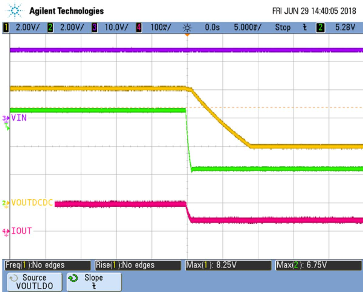
**Figure 5. The LMR33630 Tracking the Down-ramp of the LDO Voltage**
