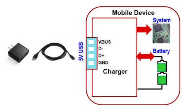
Figure 1. A Boost Charger in a 5-V USB 2S Battery System
