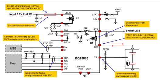
Figure 2. BQ25883 Boost Charger System Diagram
