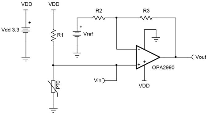
Figure 3. Temperature Sensing with PTC Circuit
