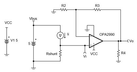
Figure 1. Single-supply Low-side Unidirectional Current-sensing Circuit
