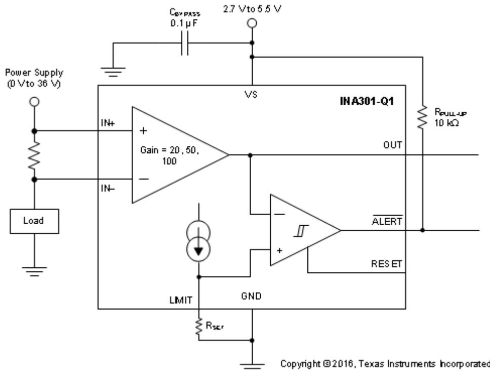
**Figure 3. INA301 Functional Block Diagram**
