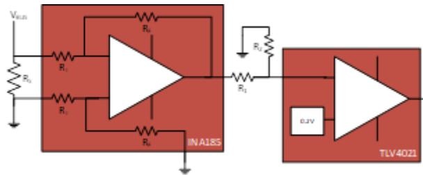
**Figure 2. Overcurrent Detection Implementation Featuring a Precision Current-sense Amplifier and Precision Comparator**
