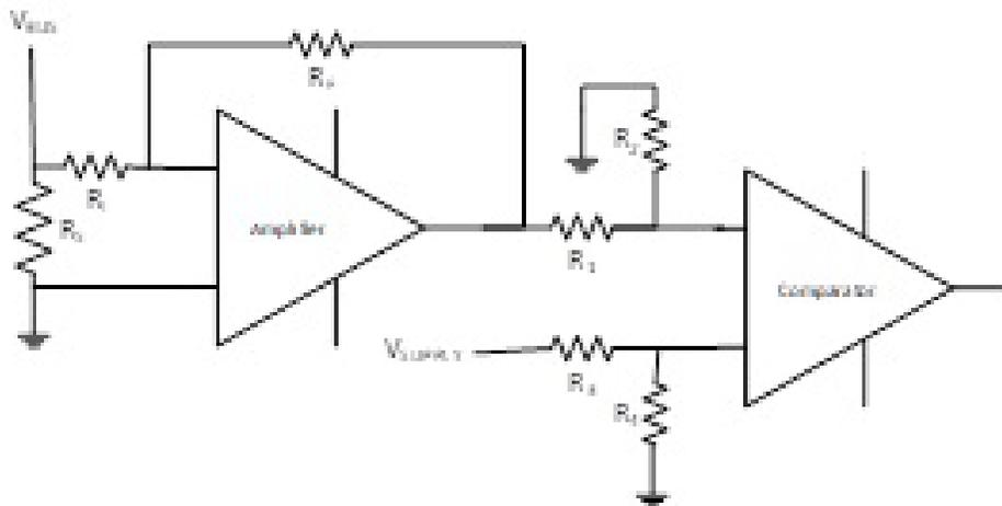
**Figure 1. Overcurrent Detection Implementation Featuring a Discrete Operational Amplifier and Comparator**
