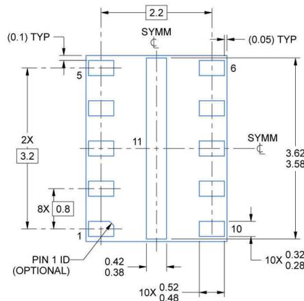
**Figure 1-2. TPSM265R1 package drawing**
