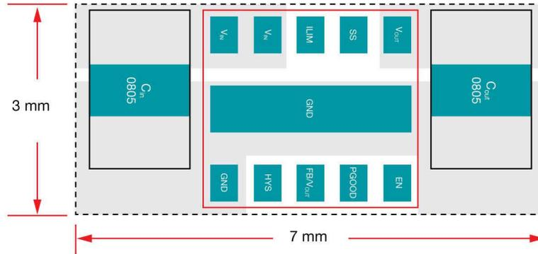
**Figure 1-3. Example layout with the [TPSM265R1](#)**
