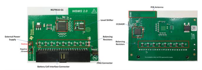
Figure 1. TI's wireless BMS architecture
