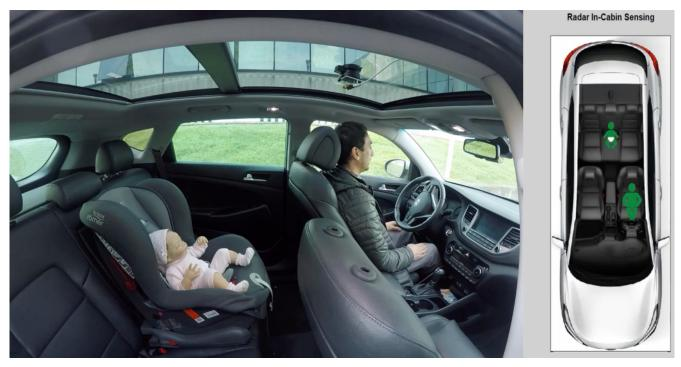
Figure 1. The detection and classification of occupants in two rows of a vehicle using TI radar (Source: Azcom Technology)
