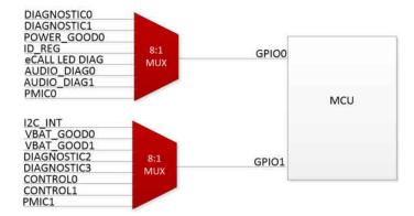
Figure 1. General-purpose input/output (GPIO) expansion with 8:1 multiplexers
