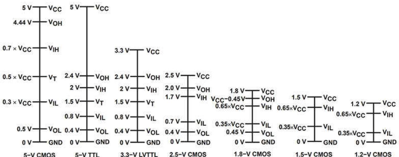
Figure 2. Standard Logic Levels
