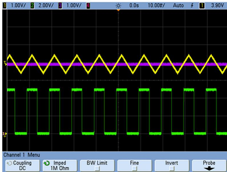
**Figure 5. LM393 Room Temperature Performance outside  $V_{CM}$**
