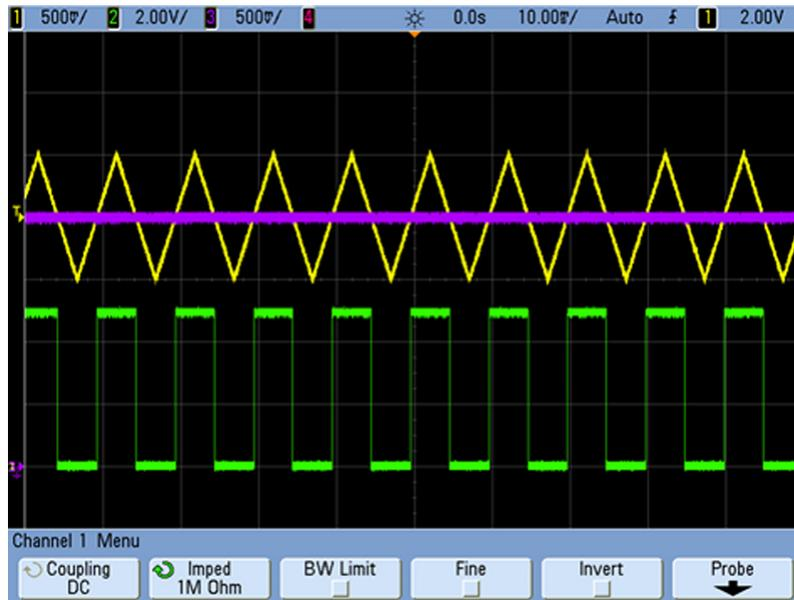
**Figure 9. LM393 Hot Temperature Performance inside  $V_{CM}$**
