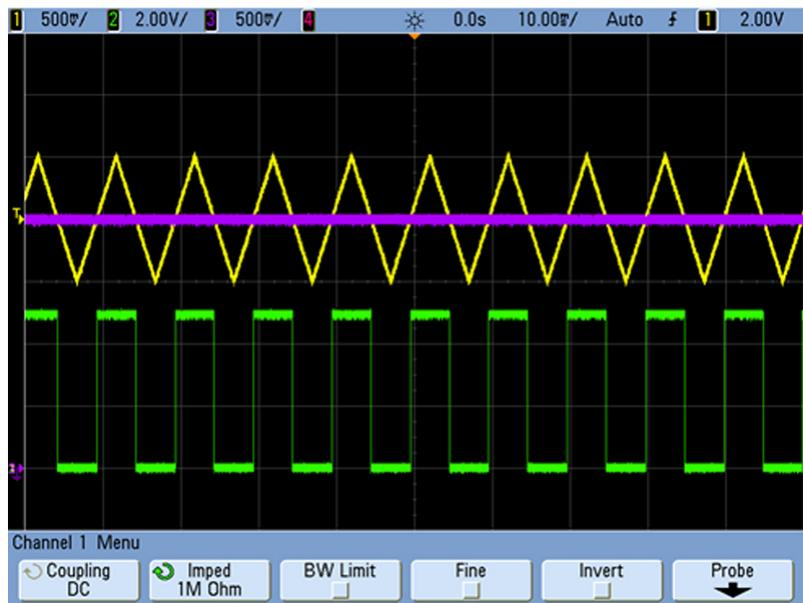
**Figure 8. LM393 Room Temperature Performance inside  $V_{CM}$**
