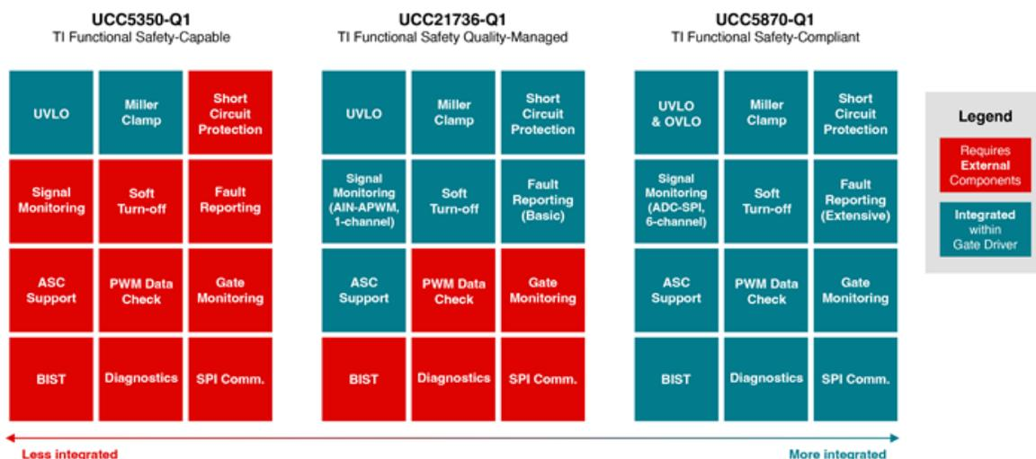
**Figure 1. A Comparison of Isolated Gate Drivers by TI Functional Safety Category and Level of Feature Integration.**
