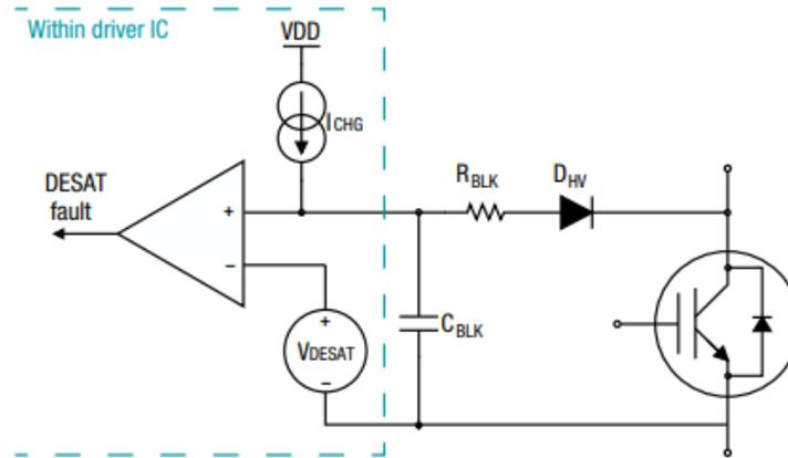
Figure 1. Typical Desat Circuit Implementation
