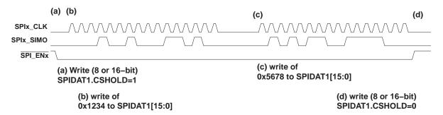
Figure 6. Workaround Assuming Halfword Writes to SPIDAT1
