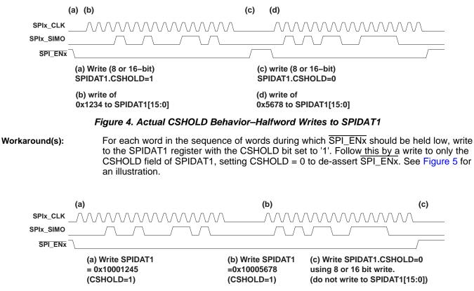
Figure 5. Workaround Assuming 32-Bit Writes to SPIDAT1 Followed by a Write Only to CSHOLD
