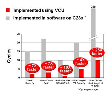
Figure 6-1. VCU Performance Improvements Compared to Software-Only Implementations
