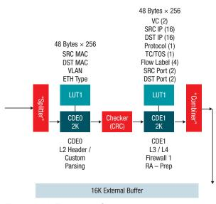
Figure 3. K2E Network Coprocessor ingress stage 0 architecture
