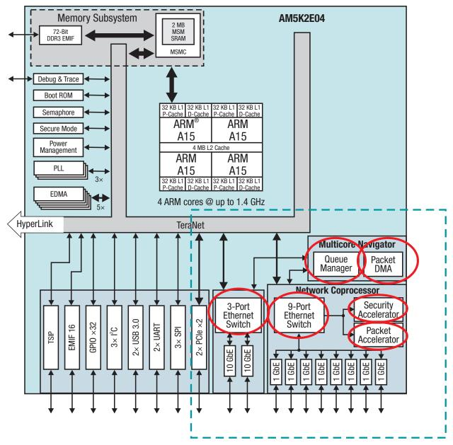
Figure 1. K2E (AM5K2E04) block diagram
