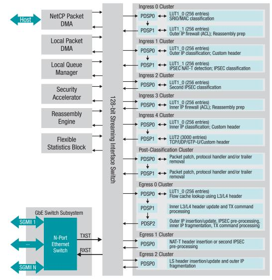
Figure 2. K2E Network Coprocessor packet accelerator
