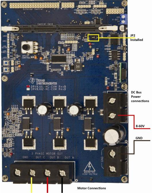
Fig2: DRV830x-HC-EVM Board Connections and Settings
