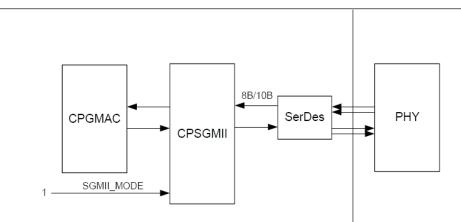
The following setup shows the CPSGMII setup for this mode of operation:
