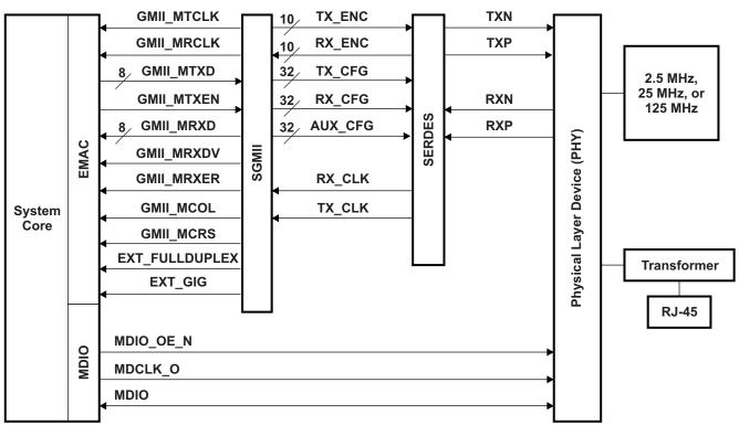
Figure 2. Ethernet Configuration with SGMII Interface
