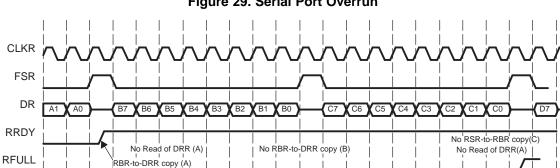
Figure 29. Serial Port Overrun
