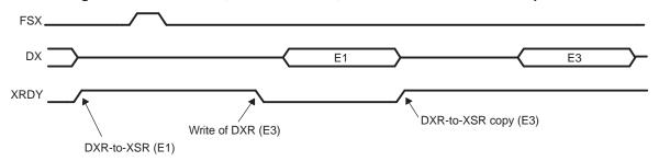
Figure 45. XMCM = 10b, XPABLK = 00b, XCER = 1010b for XMCM Operation
