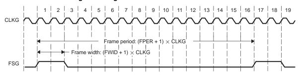
Figure 9. Programmable Frame Period and Width
