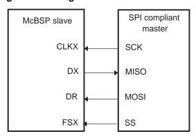
The clock stop mode (CLKSTP) of the McBSP provides compatibility with the SPI protocol. The McBSP supports two SPI transfer formats that are specified by the clock stop mode bits (CLKSTP) in SPCR. The CLKSTP bits in conjunction with the CLKXP bit in PCR allows serial clocks to be stopped between transfers using one of four possible timing variations. Figure 50 and Figure 51 show the timing diagrams of the two SPI transfer formats and the four timing variations.
