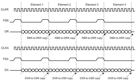
Figure 27. Maximum Frame Frequency Operation with 8-Bit Data
