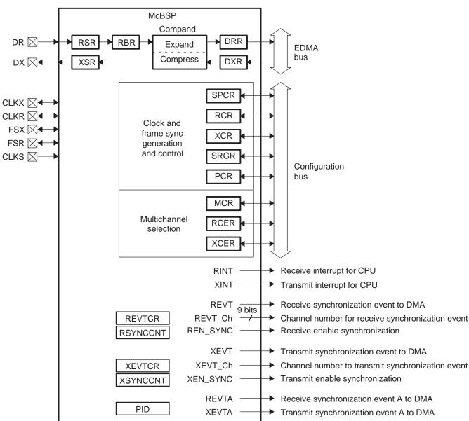
Figure 1. McBSP Block Diagram
