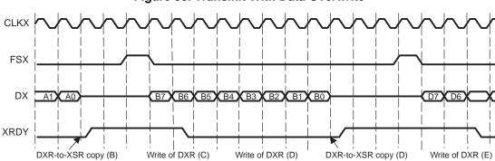
Figure 33. Transmit With Data Overwrite
