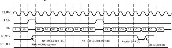
Figure 30. Serial Port Receive Overrun Avoided
