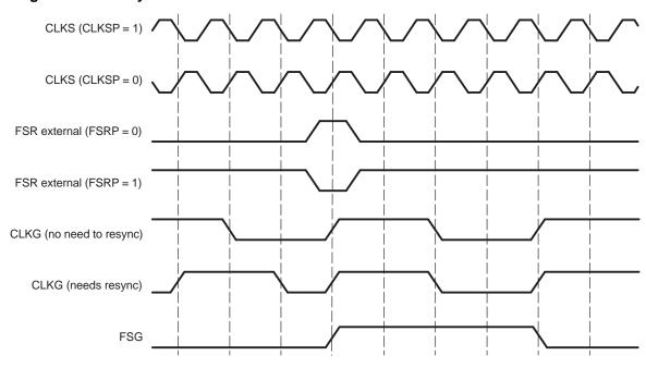
Figure 8. CLKG Synchronization and FSG Generation When GSYNC = 1 and CLKGDV = 3
