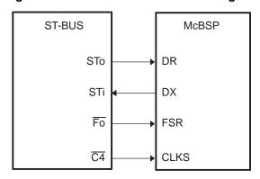
Figure 18. Double-Rate ST-BUS Clock Example
