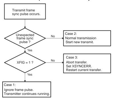
Figure 37. Unexpected Transmit Frame Synchronization Pulse
