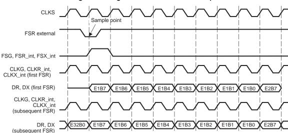
Figure 19. Single-Rate ST-BUS Clock Example
