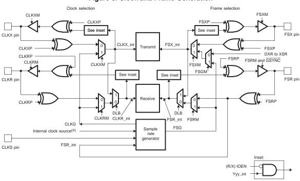
Figure 3. Clock and Frame Generation
