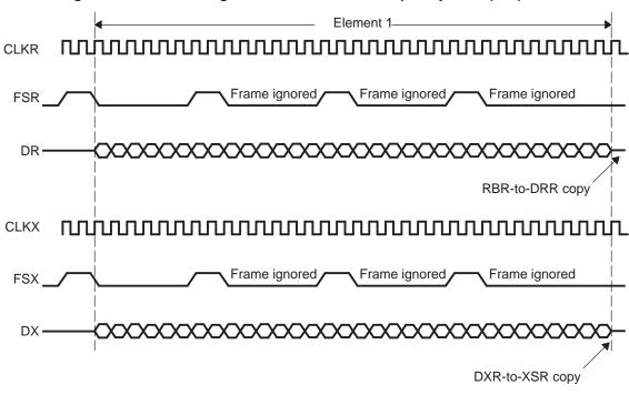
Figure 28. Data Packing at Maximum Frame Frequency With (R/X)FIG = 1
