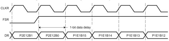
Figure 16. AC97 Bit Timing Near Frame Synchronization
