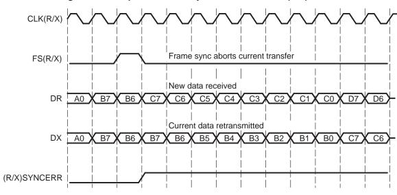
Figure 25. Unexpected Frame Synchronization With (R/X) FIG = 0
