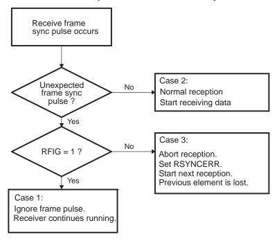
Figure 32. Unexpected Receive Synchronization Pulse
