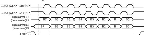
Figure 51. SPI Transfer with CLKSTP = 11b
