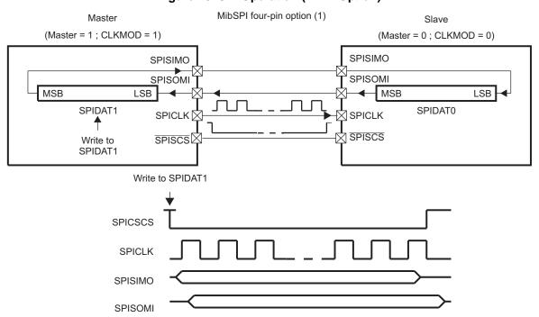
Figure 10. SPI Operation (4-Pin Option)
