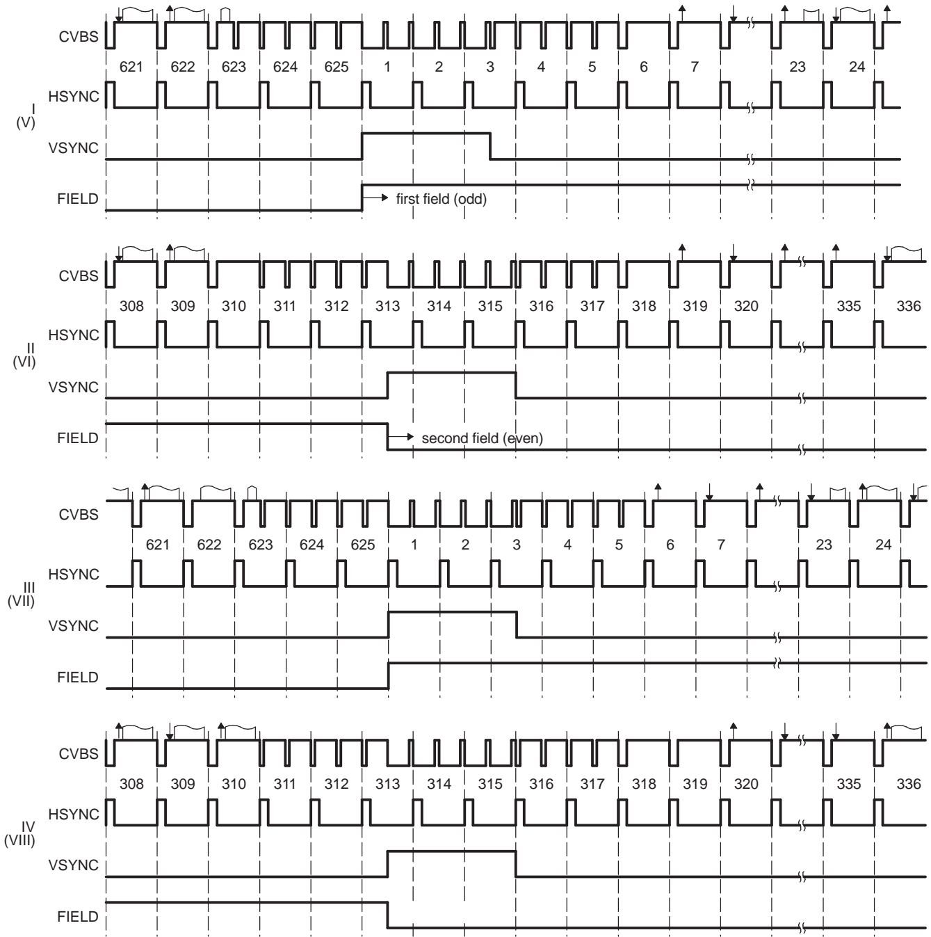
Figure 6. PAL Vertical Timing
