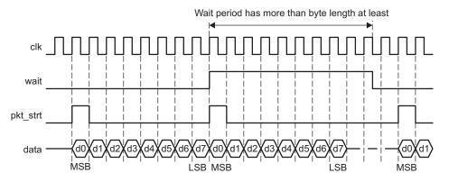
In transmitter mode, the wait signal from the external host device is detected by the TSIF module. The wait signal is latched by the pulse signal that indicates the start of a byte data (byte\_start signal for internal use). If the signal is detected by the TSIF module, the module stalls the output after a byte transfer is finished. The minimum unit of data transfer is a byte. All data with a data\_enable signal is detected by the external host device.
