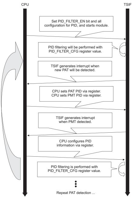
Figure 16. Processing on Semi-Automatic Mode-A of PID Filter
