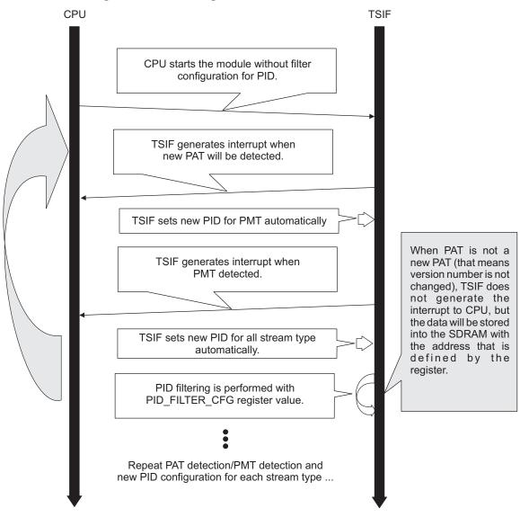
Figure 18. Processing on Full Automatic Mode of PID Filter
