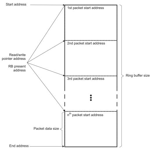
Figure 19. Ring Buffer Controller
