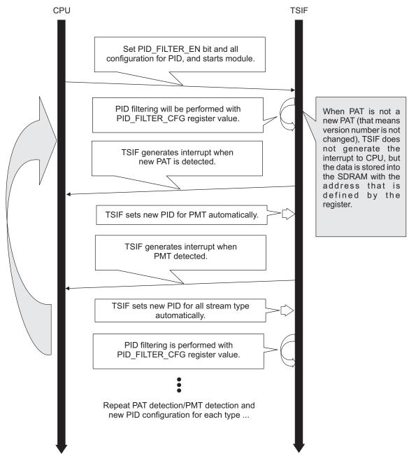
Figure 17. Processing on Semi-Automatic Mode-B of PID Filter
