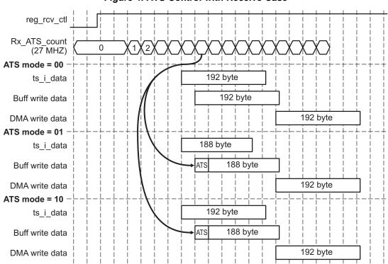
Figure 4. ATS Control with Receive Case
