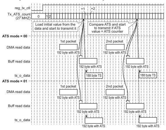
Figure 5. ATS Control with Transfer Case using Packet Data Initial Value
