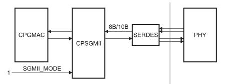
The following setup shows the CPSGMII setup for this mode of operation:
