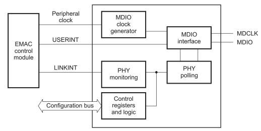
Figure 9. MDIO Module Block Diagram
