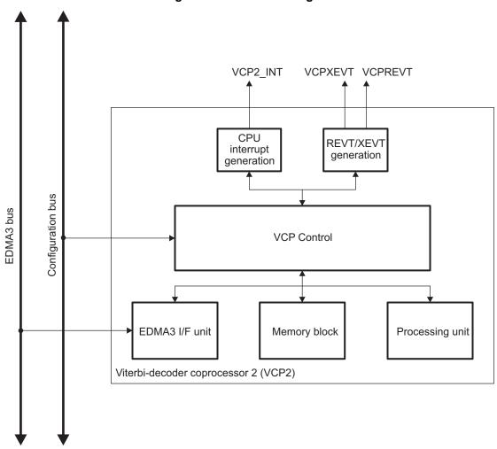
Figure 3. VCP2 Block Diagram
