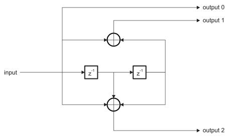
Figure 1. Convolutional Encoder Example Block Diagram
