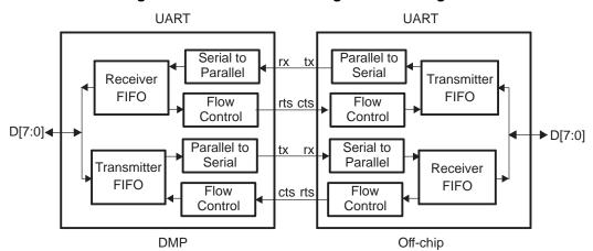
Figure 5. UART Interface Using Autoflow Diagram
