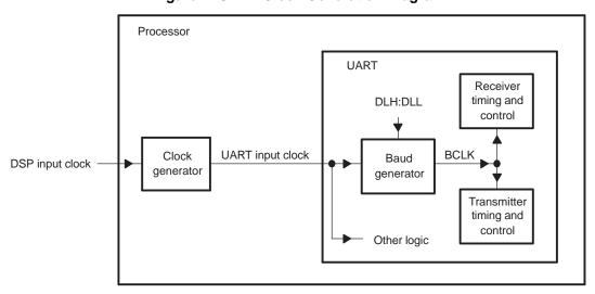
Figure 2. UART Clock Generation Diagram
