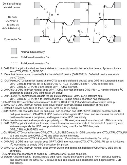
R. OMAP5912 USB device controller sees and responds appropriately to USB reset, set feature of the B\_HNP\_ENABLE feature, enumeration, and normal USB bus activity.
