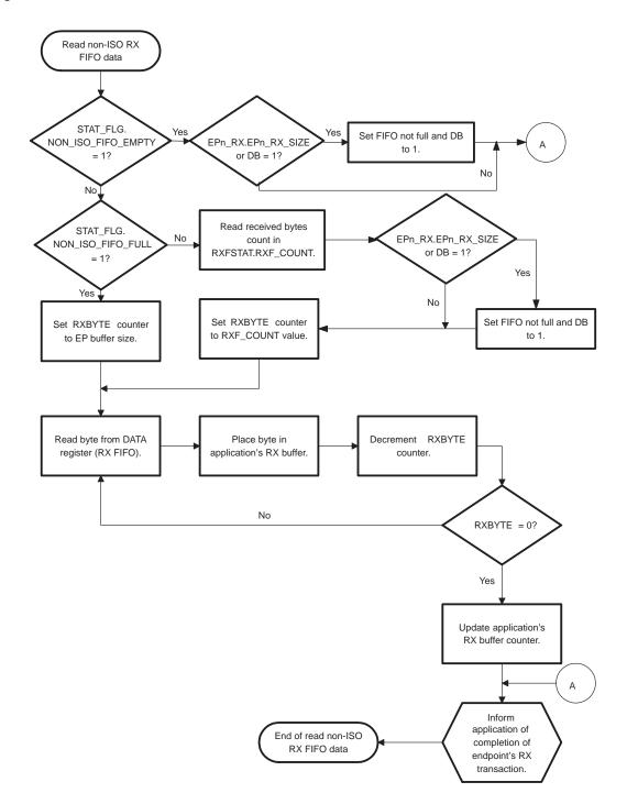
Figure 31. Read Non-Isochronous RX FIFO Data Flowchart
