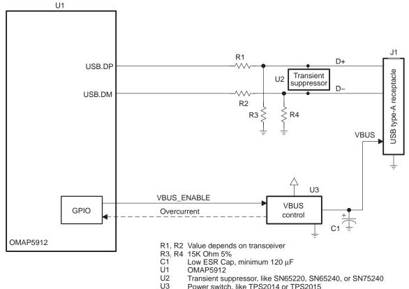
USB Host Connections Using the OMAP5912 Integrated USB Transceiver Figure 66.
