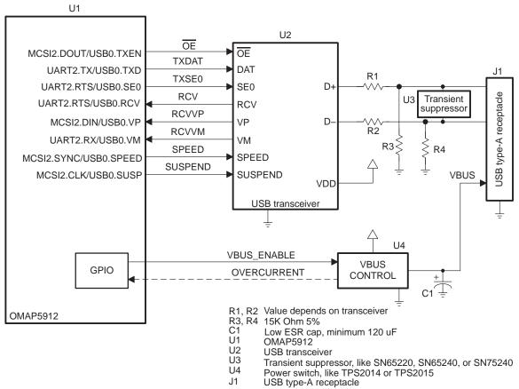
USB Host Connections on USB Alternate Pin Group 2 Using 6-Wire Figure 75. Transceiver
