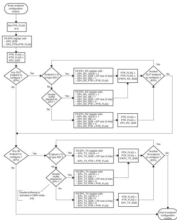
Figure 12. Endpoint Configuration Routine
