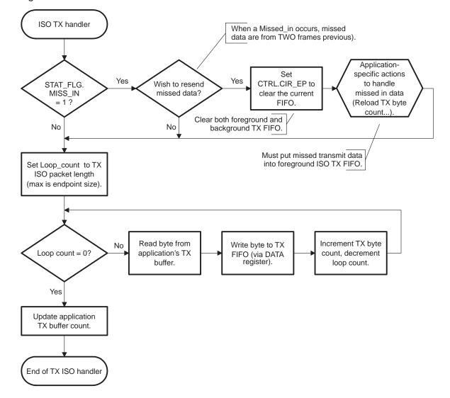
Figure 36. Write Isochronous TX FIFO Data Flowchart
