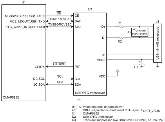
Figure 60. OTG on USB Pin Group 1 Using 3-Wire OTG Transceiver
