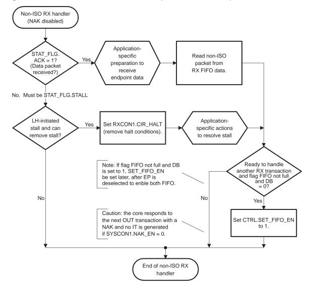
Figure 30. Non-Isochronous Non-Control Endpoint Receive Interrupt Handler
