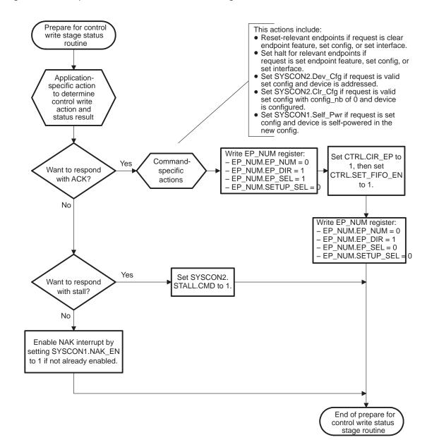
Figure 19. Prepare for Control Write Status Stage Routine
