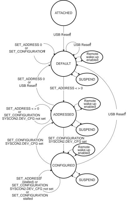
Behavior not specified by USB 1.1 specifications (see chapter 9) USB reset generates two interrupts (when USB reset is asserted and then when USB reset completes). <sup>‡†</sup> No interrupt is asserted by the core for tansitions shown with dashed lines.
