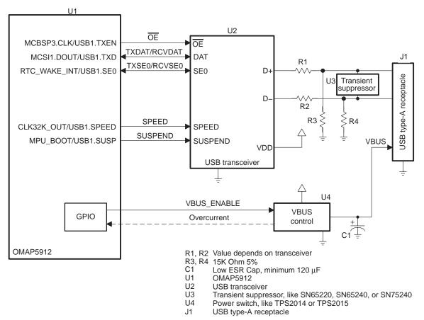
Proper initialization of the OMAP5912 device to support this mode of operation requires proper setting of the top-level pin multiplexing for these pins:
