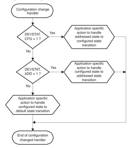
Figure 25. Configuration Changed Handler
