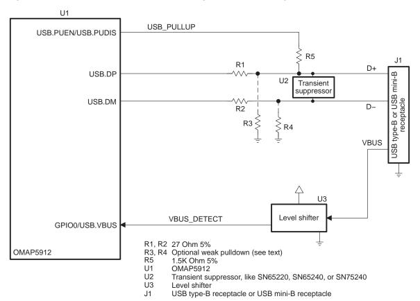
Proper initialization of the OMAP5912 to support this mode of operation requires proper setting of the top-level multiplexing for USB.DP and USB.DM (see Table 74) and selection of an HMC\_MODE value that routes the USB device controller to pin group 0 (see Table 73). OTG\_SYSCON\_1. USB0.TRX\_MODE must be set to 3 to allow proper operation of the integrated USB transceiver.
