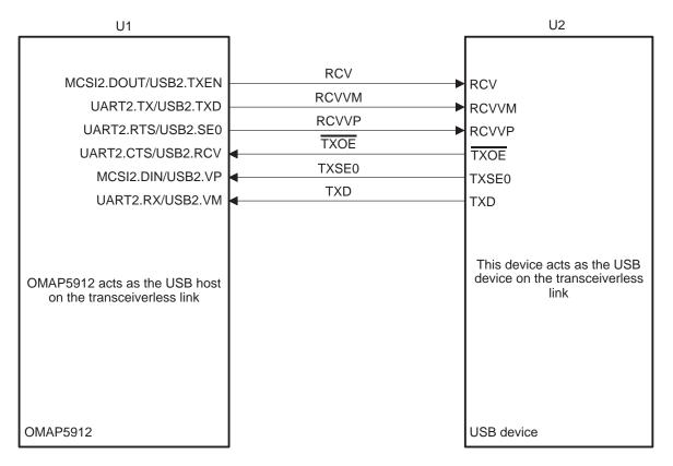
Proper initialization of the OMAP5912 device to support this mode of operation requires proper setting of the top-level pin multiplexing for these pins:
