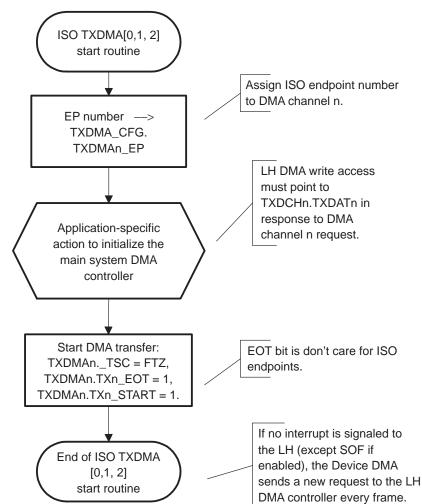
Figure 45. ISO TX DMA Start Routine
