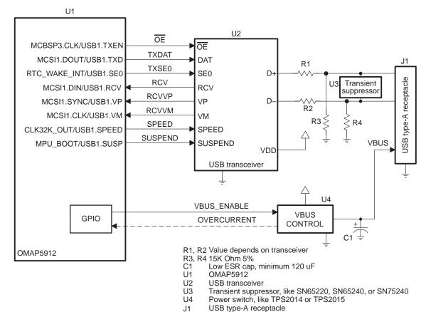
Figure 69. USB Host Connections on USB Pin Group 1 Using 6-Wire OTG Transceiver
