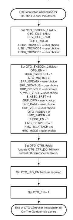
Figure 48. OTG Controller Initialization When Implementing an OTG Dual-Role Device
