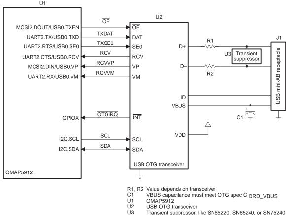
OTG on USB Alternate Pin Group 2 Using 6-Wire OTG Transceiver Figure 65.
