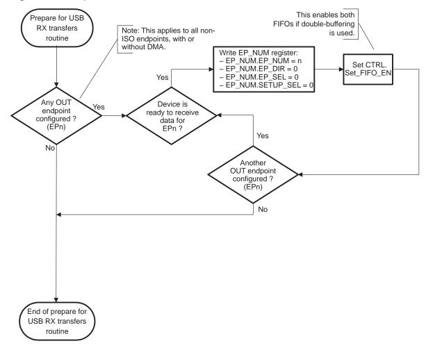
Figure 13. Prepare for USB RX Transfers Routine
