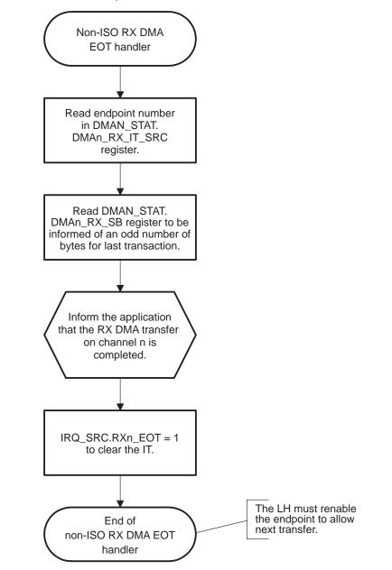
Figure 39. Non-ISO RX DMA EOT Interrupt Handler
