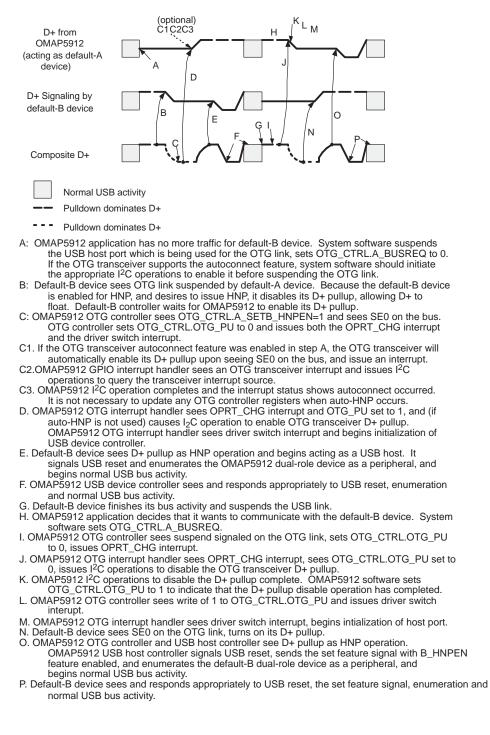
Figure 58 shows the typical events that occur when OMAP5912 acts as an OTG default-B dual-role device and transitions from acting as a B-peripheral to acting as a B-host via HNP, and then transitions back to acting as a B-peripheral via HNP.
