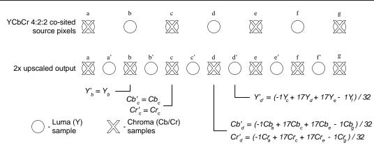
Figure 16. Video Output 2x Scaling
