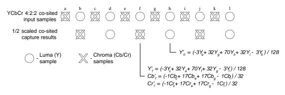
Figure 11. Video Input 1/2 Scaling
