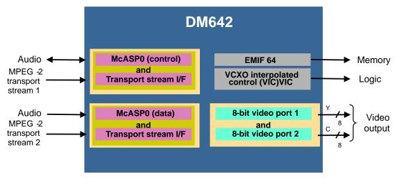
Figure 22. Set-Top Box Application Using a DM642
