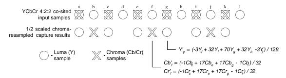
Figure 12. Video Input 1/2 Scaling With Chrominance Resampling
