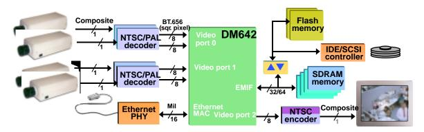
Figure 23. Networked DVR System Using a DM642
