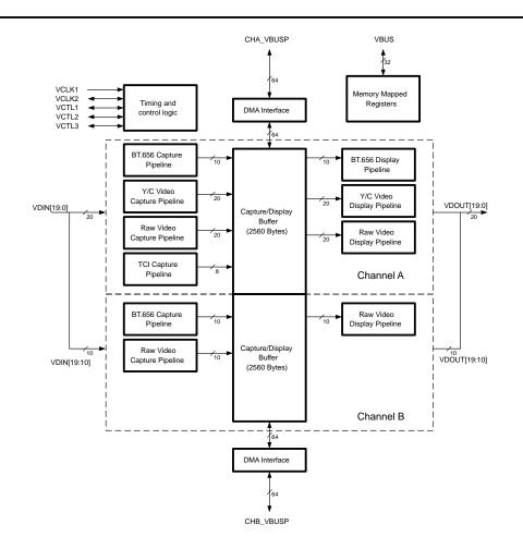
Figure 6. Video Port Block Diagram
