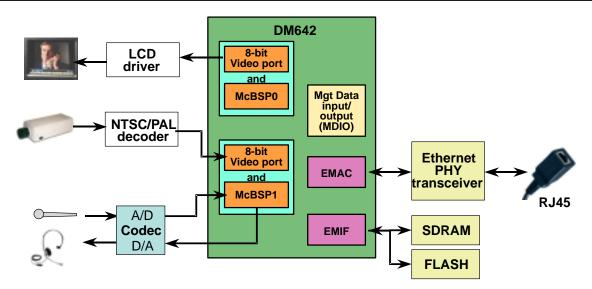
Figure 21. DM642 Based Video IP Phone
