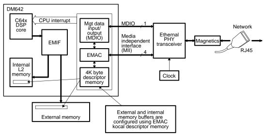
Figure 19 shows DM642 networking using the EMAC and MDIO.
