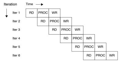
The memory system's coherence directly supports this programming technique. A system of snoops and invalidates (as discussed in section 5.4.2) keeps L2 SRAM and L1D in sync without programmer intervention. In the context of this example, the memory system performs the following operations in response to each of the numbered steps in Figure 25.
