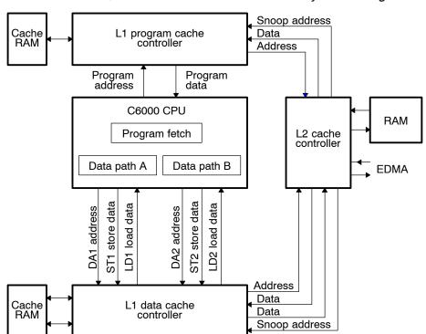
Figure 2. TMS320C621x/C671x Two-Level Internal Memory Block Diagram
