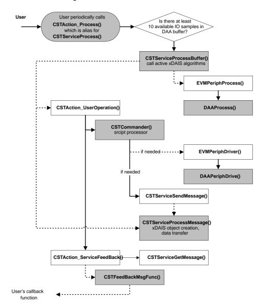
Figure 6-5. Schematic Diagram of CST Periodic Thread Call Tree
