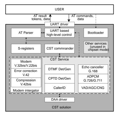
Figure 6-1. CST Framework Controlled via AT Command Parser
