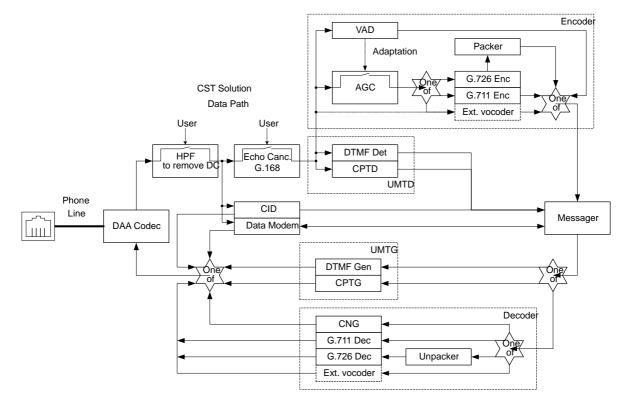
The user can control the way components are connected inside the CST framework and what components are currently active via AT commands or, in flex mode, via messages to one of CST control layers.
