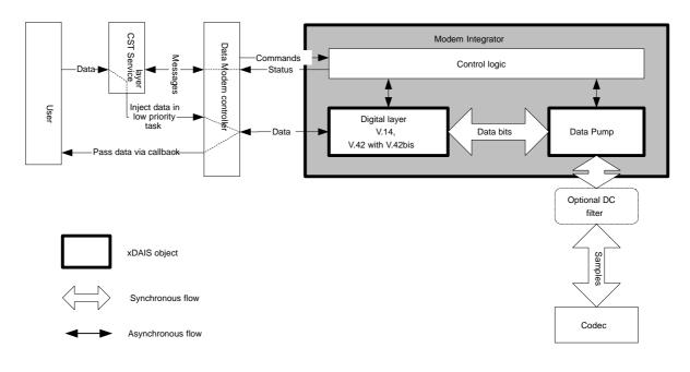
As it has been mentioned, the modem passes the decoded data through a callback function. Besides this data callback function, there are two other (optional) callback functions to be implemented by user.
