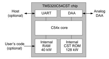
The most generic hardware setup for CST Chip is shown in Figure 3-2.
