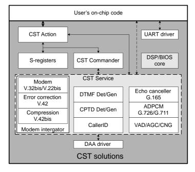
Figure 6-2. CST Framework Controlled via CST Action Layer
