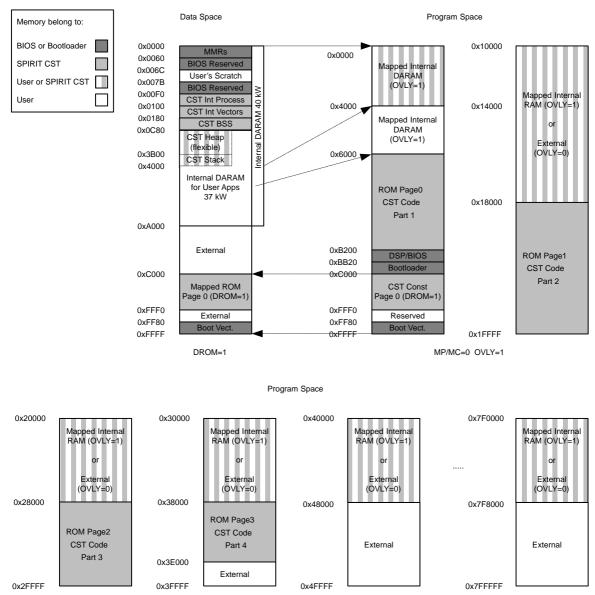
In chipset mode, if update patch is not loaded, CST uses only 16 kW of internal RAM of C54CST chip (from 0x60 to 0x3FFF). After update patch is loaded, CST starts using all 40 kW of available internal RAM.
