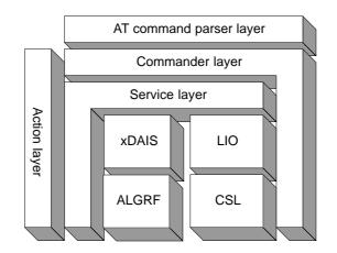
CST Framework has two alternative top layers and therefore, two alternative top-level interfaces.
