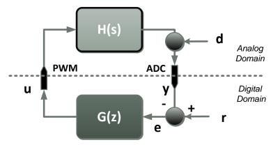
Figure 4. Digitally Controlled Control System
