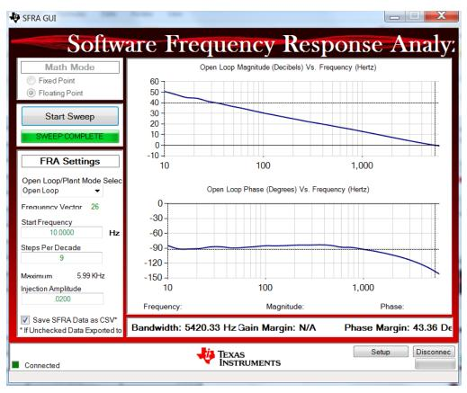
Figure 12. SFRA Plot of Current Loop With Higher Bandwidth Design
