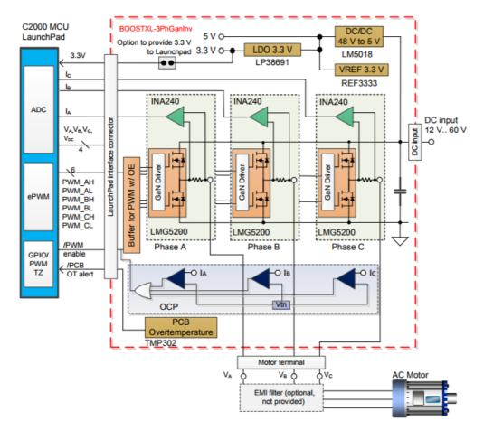
Figure 6. BOOSTXL-3PHGANINV Functional Block Diagram
