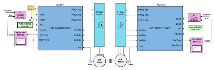
Figure 10. Level 6 Incremental System Build Block Diagram
