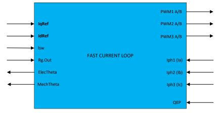
Figure 3. Fast Current Loop (FCL) Library Block Diagram
