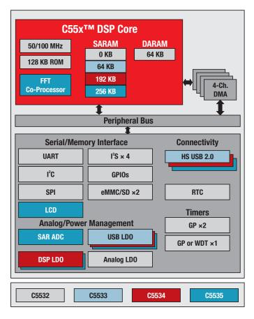
industry's lowest power consumption. The C553x generation of DSPs delivers up to six times lower power consumption compared to the nearest DSP competitor (active power less than 0.15 mW/mHz at 1.05V and standby power less than 0.15 mW), allowing extremely power-efficient portable devices.
