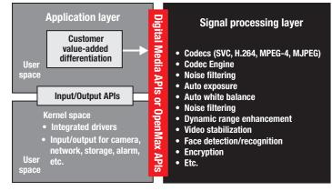
TMS320DMxx-based IP Camera reference design software
