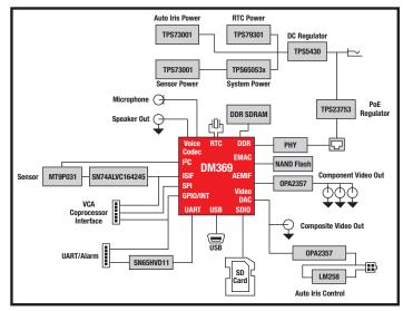
▲ IP camera reference design block diagram: TMDSIPCAM369X104
