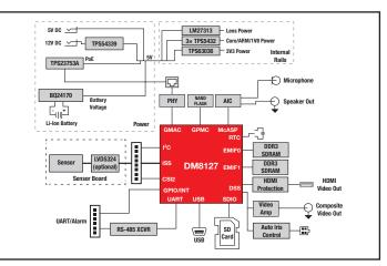
🔺 DM8127 IP camera reference design block diagram: TMDXIPCAM8127J3
