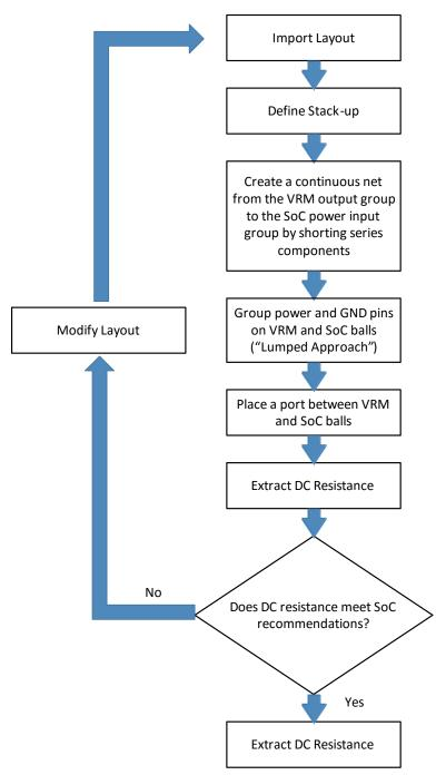
Figure 2. DC Resistance Extraction Flow
