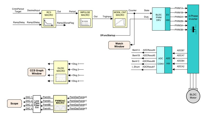
Level 2 verifies the open loop motor operation and current measurement.
