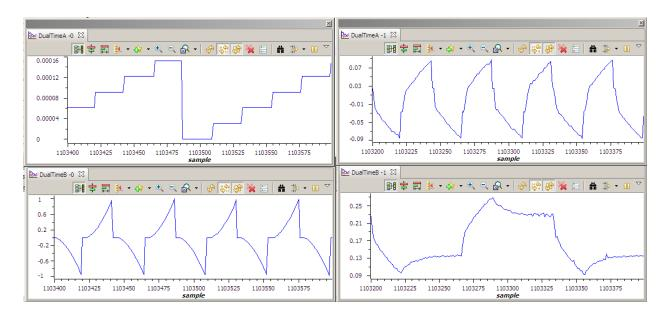
Figure 12 Graph Windows for Build Level 8 (a) mod6 counter, (b) V\_int, (c) Vphase and (d)Vag
