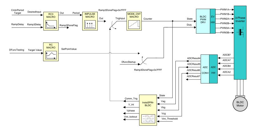
Level 5 verifies the closed loop motor operation based on InstaSPIN-BLDC and the resulting commutation trigger points.
