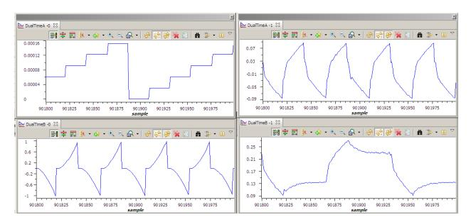
Figure 11 Graph Windows for Build Level 7 (a) mod6 counter, (b) V\_int, (c) Vphase and (d)Vag
