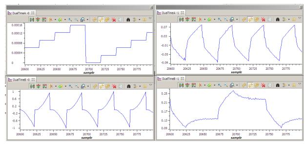
Figure 9 Graph Windows for Build Level 5 (a) mod6 counter, (b) V\_int, (c) Vphase and (d)Vag
