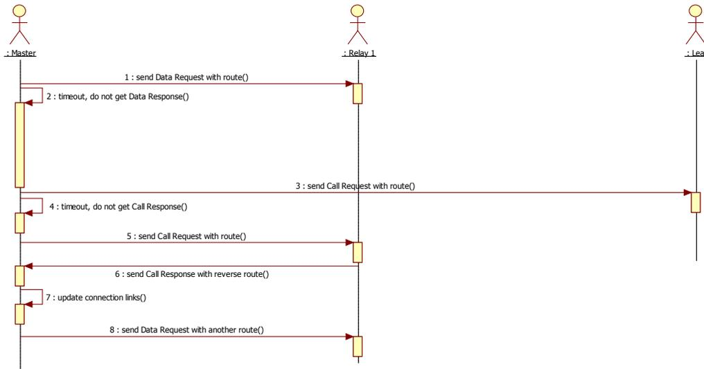
**Figure 7. Data Request Failure, Maintenance, Sequence Chart**
