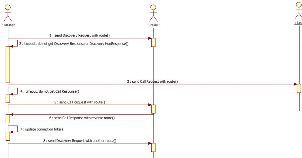
**Figure 5. Discovery Failure, Maintenance, Sequence Chart**
