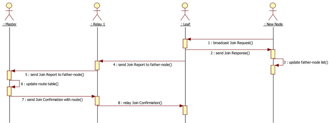
**Figure 8. Join With Response, Sequence Chart**
