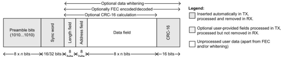
**Figure 1. Physical Frame Format**
