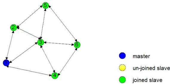
**Figure 17. All Nodes Discovered for New Connections**
