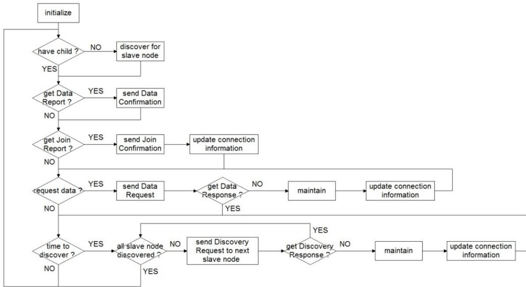
**Figure 11. Flow Chart of Master Node**
