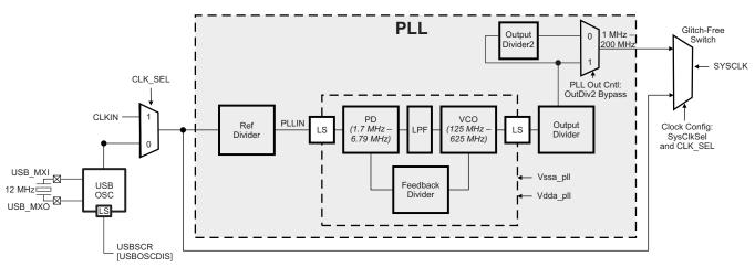
Figure 2. System PLL Block Diagram
