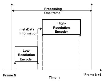
Figure 2. Sequential Operation of the Low- and High-Resolution Encoders
