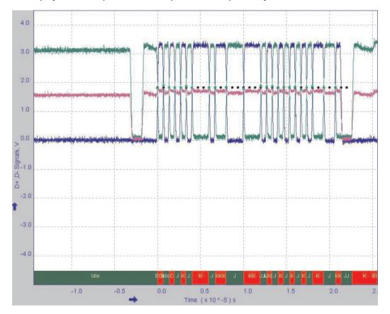
Figure 25. Low-Speed Waveform Plot
