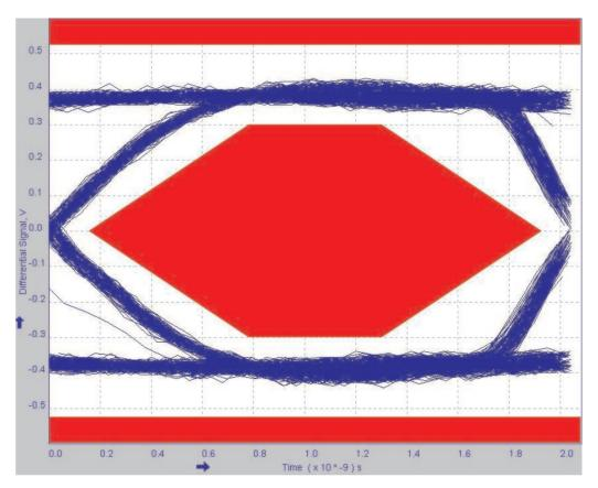
Figure 3. Downstream Eye Diagram
