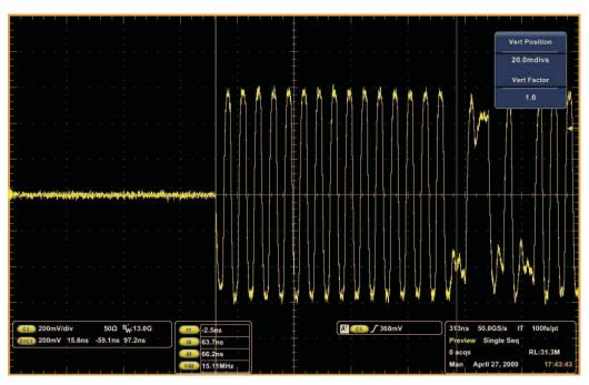
Figure 9. Status Stage of a GET DEVICE DESCRIPTOR Transaction SYNC Field of the Token Packet
