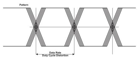
Figure 6. Duty Cycle Distortion (DCD)
