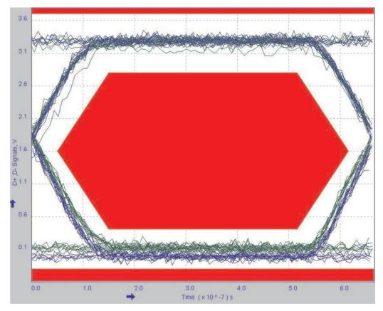
Figure 26. Low-Speed Eye Diagram
