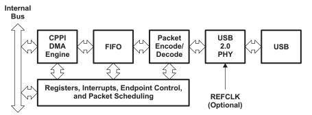
Figure 1. USB Functional Block Diagram
