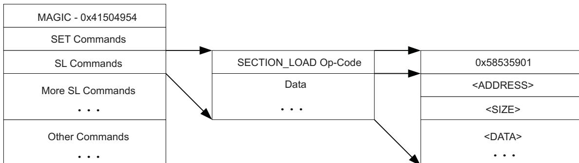
**Figure 7. Structure of Section Load Command**
