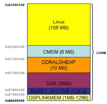
Figure 2. Example Memory Map Plan After Calculations
