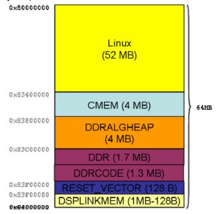
Figure 4. Resulting Memory Map After Splitting DDR
