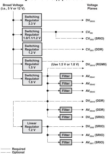
Figure 8. Power Supply Generation
