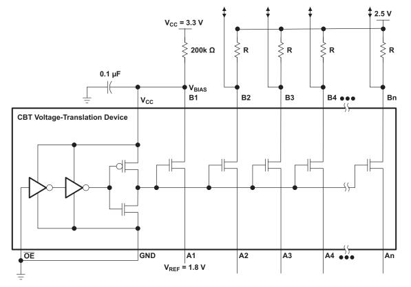
Figure 14. RGMII Voltage-Level Translation Circuit
