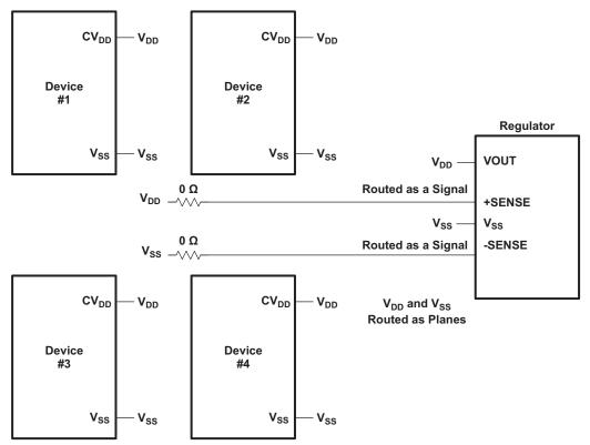
Figure 11. Multiple DSP Remote Sense Connections
