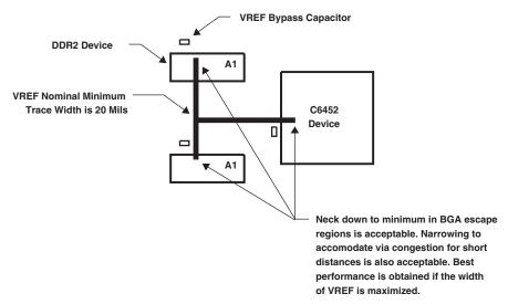
Figure 4. VREF Routing and Topology
