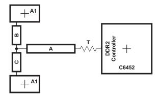
Figure 5. CK and ADDR\_CTRL Routing and Topology
