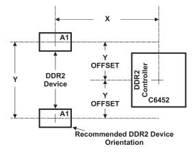
Figure 2. C6452 and DDR2 Device Placement
