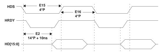
Figure 1. Multiplexed Read Timing With Auto-Increment
