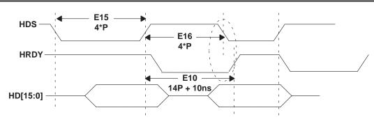
Figure 2. Multiplexed Write Timing With Auto-Increment
