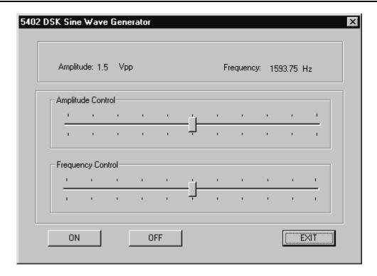
You can press the buttons and move the controls to obtain similar results as those given by the console version. Both programs communicate with the target using function calls to evmdsk54x.dll.
