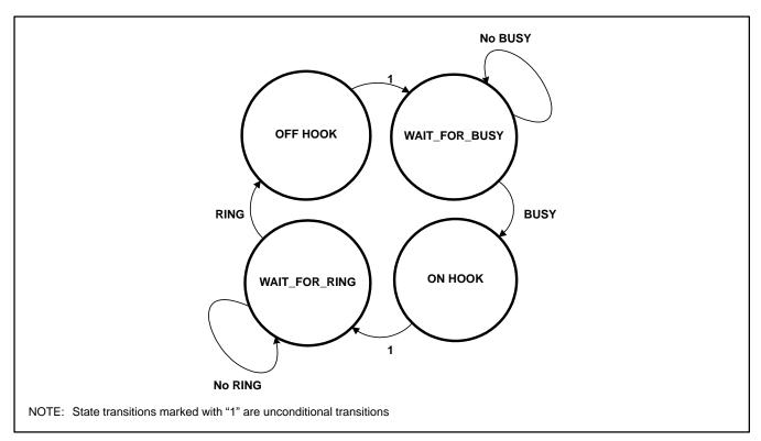
Figure 3. OFF/ON HOOK Processing
