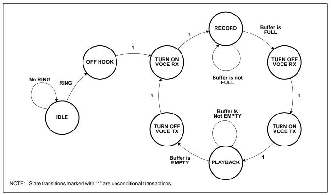
Figure 5. Recording and Playback
