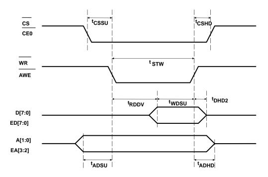
Figure 9. CS4231A Parallel Interface Write Timing
