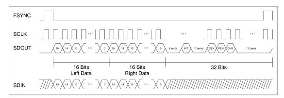
Figure 2. CS4231A 64-bit Enhanced Mode Serial Timing
