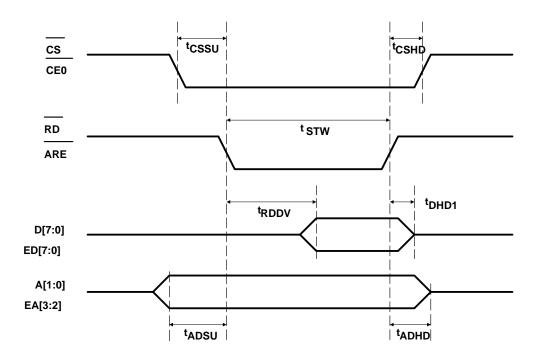
Figure 8. CS4231A Parallel Interface Read Timing
