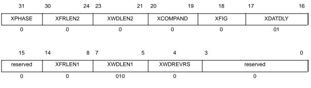
Figure 4. Transmit Control Register (XCR)
