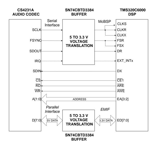
Figure 1. TMS320C6000 Interface to the CS4231A Multimedia Audio Codec
