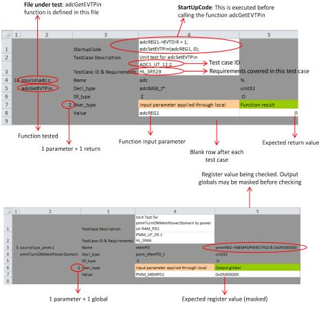
Figure 16. Examples of a Test Case
