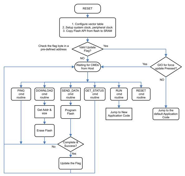
Figure 6. CAN Bootloader Flowchart
