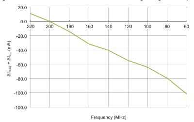
Figure 3. Current Reduction Versus HCLK on RM48L950
