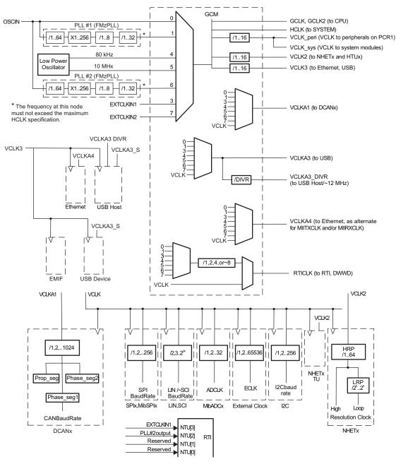
Figure 2. Clock Domain Diagram
